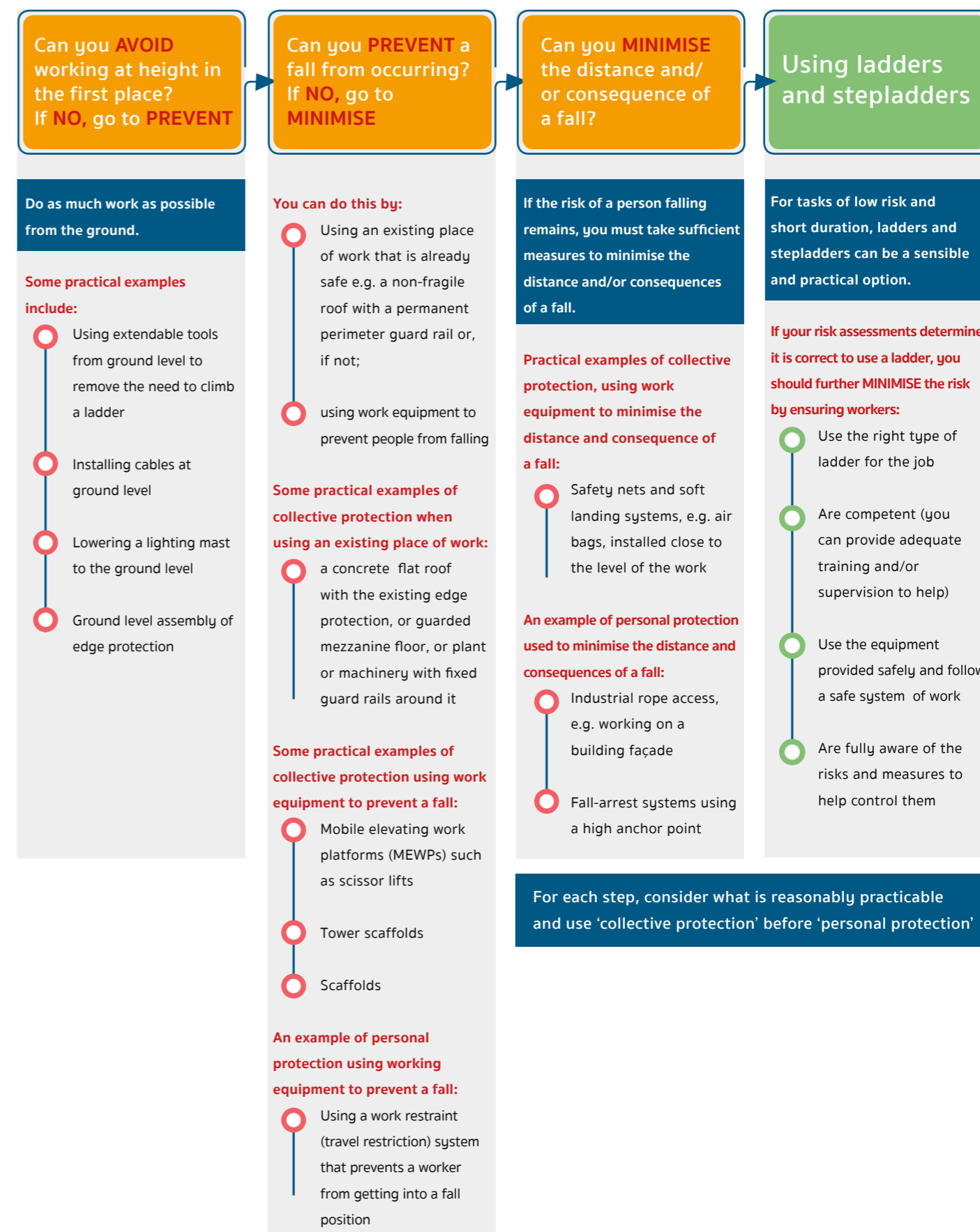
Figure 1 The Work at Height Hierarchy of measures – INDG 401 – Short Guide to Work at Height, HSE
